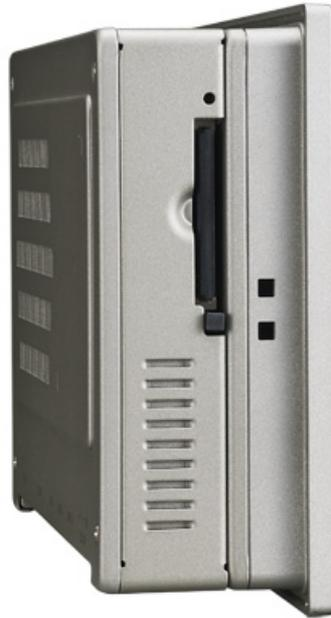
**Figure 2.2 Install CFast Memory Card**
