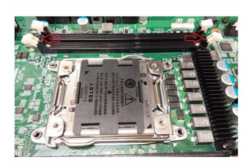
Align the memory module with the slot. When inserted properly, the memory slot locking levers lock automatically onto the indentations at the ends of the module. Follow the recommended memory population table to install the other memory modules.
