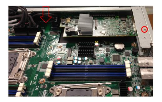
4. Install the mini-SAS HD cable into the expansion card.
