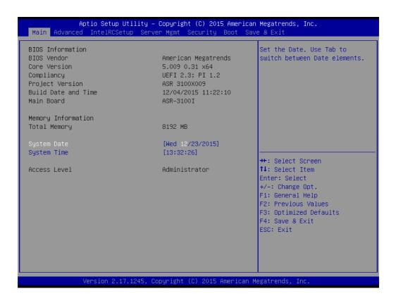
AMI's BIOS ROM has a built-in Setup program that allows users to modify the basic system configuration. This type of information is stored in battery-backed up CMOS so it retains the Setup information when the power is turned off.
