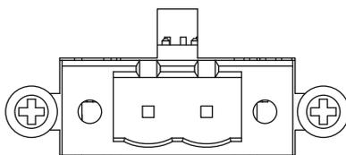
Figure 2.10 Remote Power Connector
