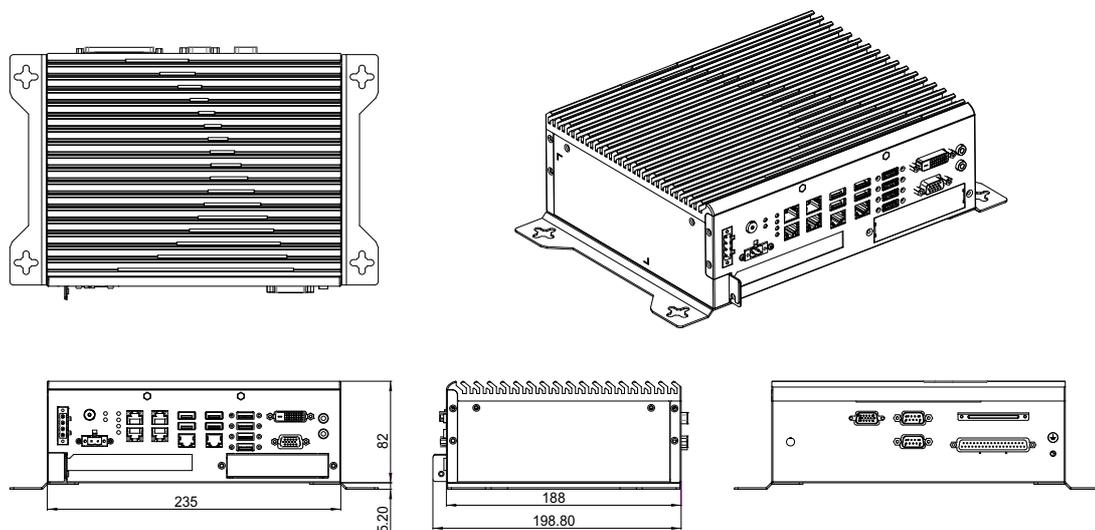
Figure 1.1 AIIS-5410P Mechanical Dimension Drawing
