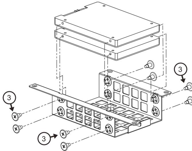
3. Secure the 4xHDD screws (P/N:1930002235)
