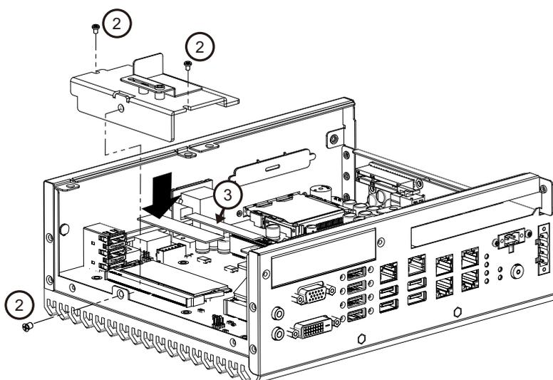
2. Undo 3 screws to remove the memory thermal cover.
