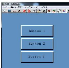
In this case, the button can choose by using cursor up/down key. So windows screen controllable. For example, if press "Down Arrow" key from above screen, the button can be chosen.
