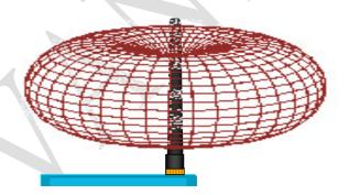
The modules without power amplifier use a build-in antenna inside the module. The build-in antenna is shown as a white bar on the left figure below. Its antenna pattern is also looks like a doughnut which vertical to antenna. The modules including: ADAM-2031Z, ADAM-2051Z, and ADAM-2017Z
