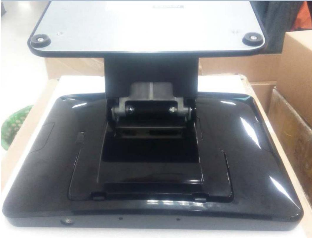
2. 拆下硬盘上方的塑料盖子 Remove the plastic cover
