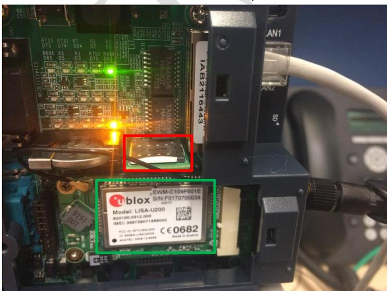
The red block indicates the position where the 3G SIM card is installed.
