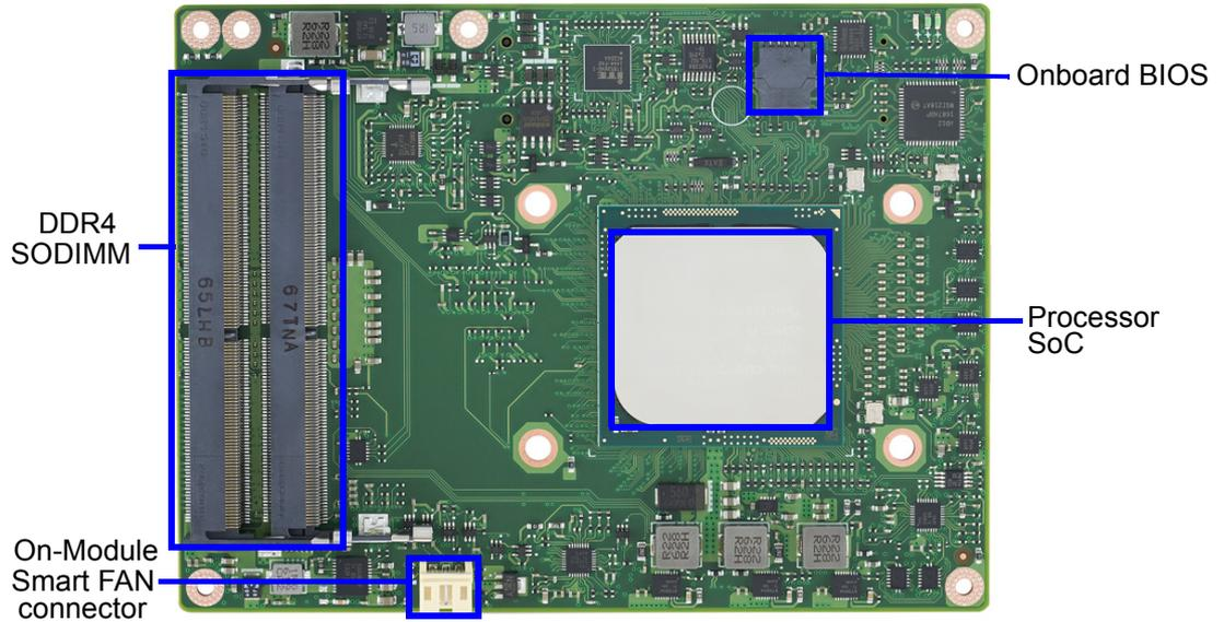
Figure 2.1 Board Chips Identify - Front
