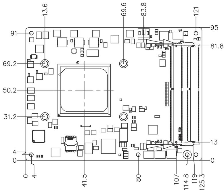
**Figure 2.3 Board Mechanical Drawing - Front**
