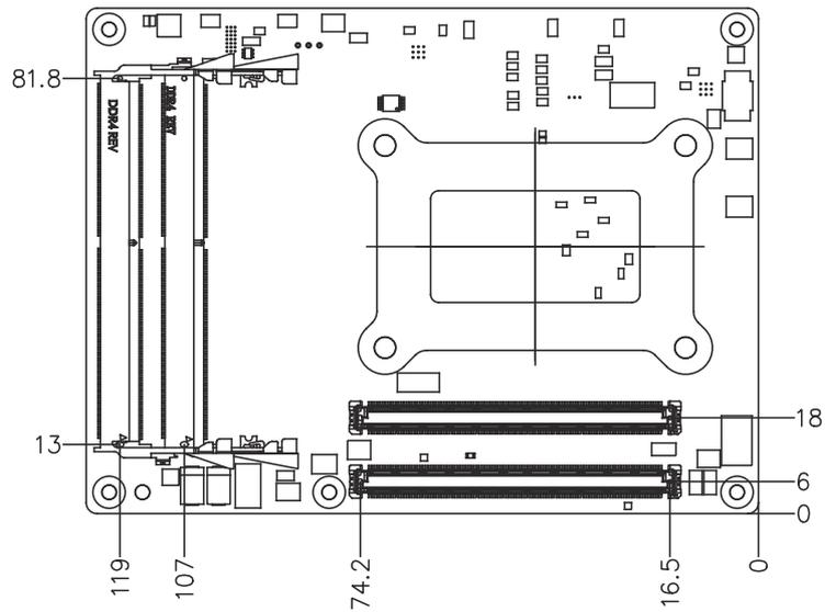
**Figure 2.4 Board Mechanical Drawing - Back**
