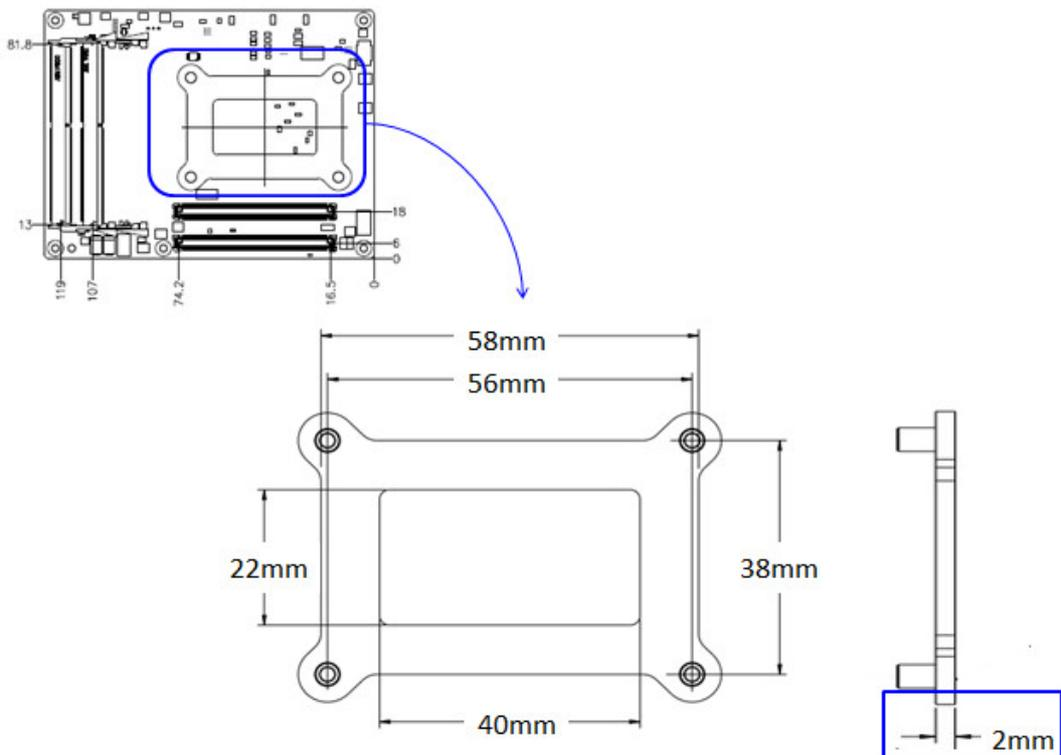
**Figure 2.8 Backplane of Optional Thermal Solution**
