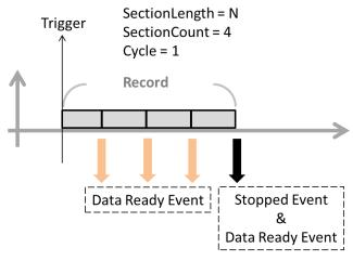
This is a function acts like the burst function of function generator. The acquisition would be stopped automatically right after the last DataReady event is raised. A start command should be entered in order to initiate next acquisition.
