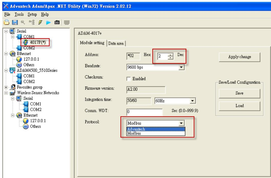
The module will automatically appear in the left tree under the serial port it is connected to.
