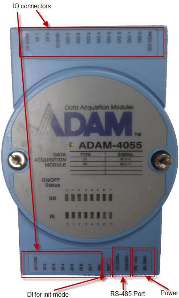
The modules contain a RS-485 port. It only has the data+ and data- connectors. If you want to connect it to an RS-232 port on your computer
