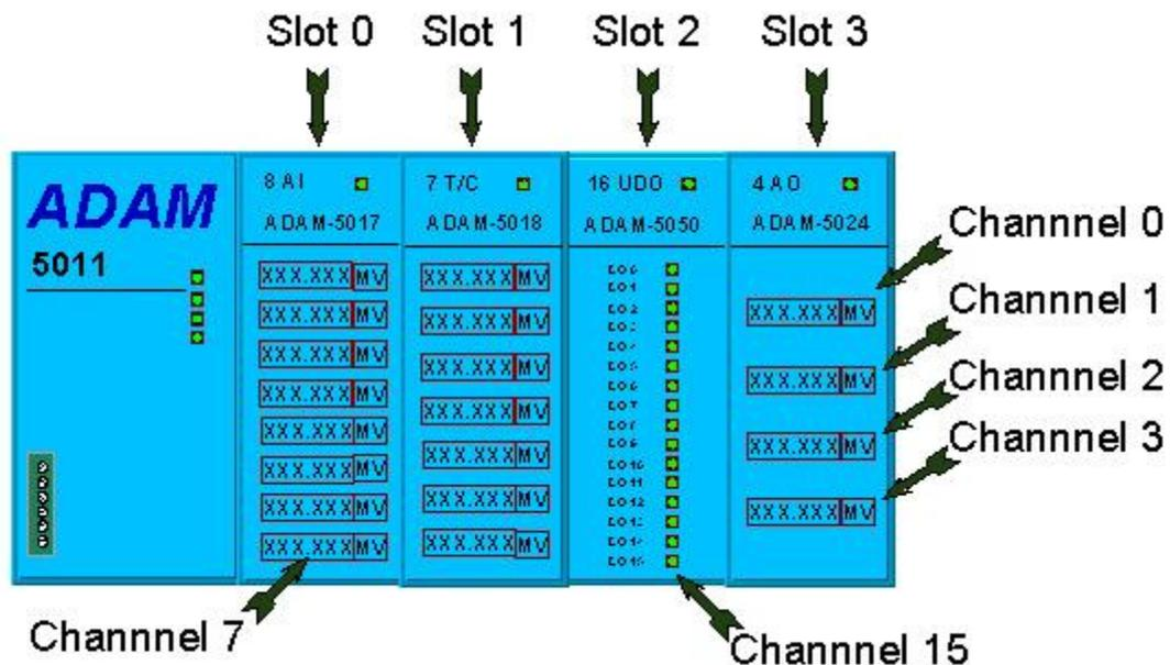
This example is to configure 4 Blocks that represent the above drawing of a ADAM 5011 processor rack, with 4 IO Modules: 5017, 5018, 5051 and 5024 in slots 0 to 3 respectively.
