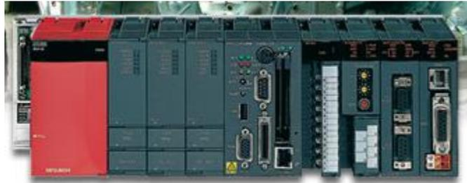
The MitsuQ driver will connect and read data directly from the PLC using the Ethernet port. The driver is listed in the TCP/IP drivers.
