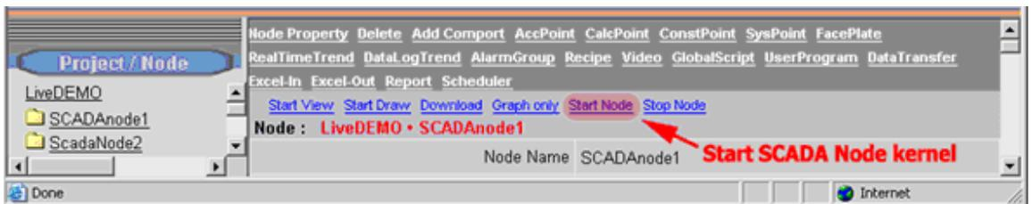
Figure 4.34 - Start SCADA Node kernel remotely via the Project Manager
