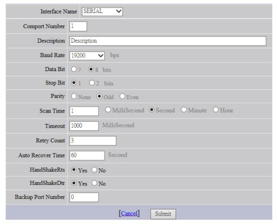
Figure 2.1 Serial Comport properties
