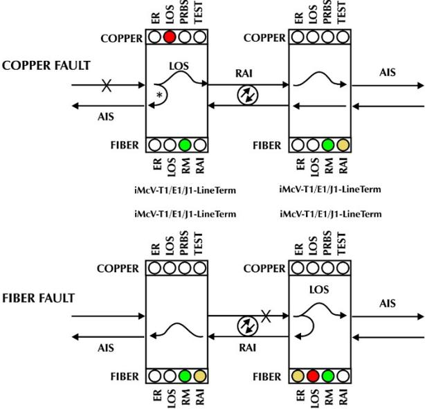
\*DIP Switch S3-7 must be set to ON for Fault Loopback to operate as illustrated.
