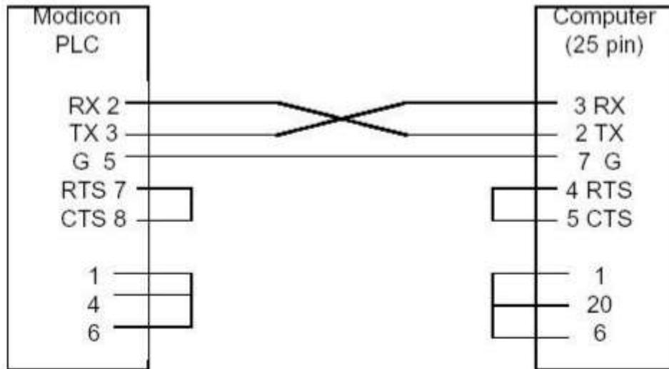
Figure 1.2 RS232-Modicon 984 Cabling Diagram (25 pin COM Port)
