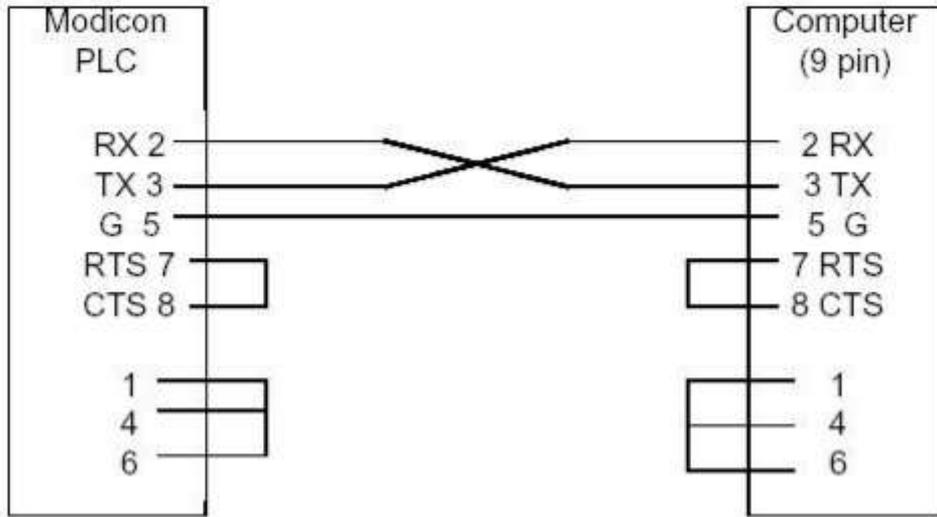
Figure 1.1 RS232-Modicon 984 Cabling Diagram (9 pin COM Port)
