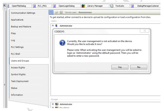
It means user management(Device User Logon) is needed whenever IDE log into RTE. Reference: <a href="https://help.codesys.com/webapp/">https://help.codesys.com/webapp/</a> cds handling user management on plc;product=codesys;version=3 <a href="mailto:5.13.0">.5.13.0</a>
