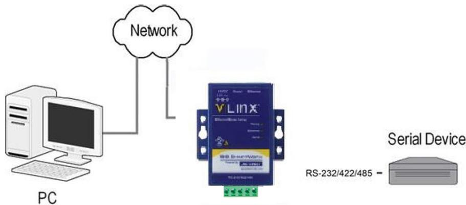
Figure 11. BB-MESP211T Connections
