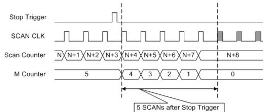
Delay to Stop Trigger ( M = 5 )
