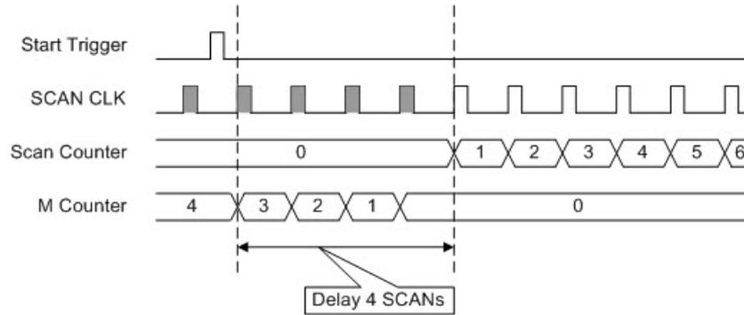
Delay to Start Trigger ( M = 4 )
