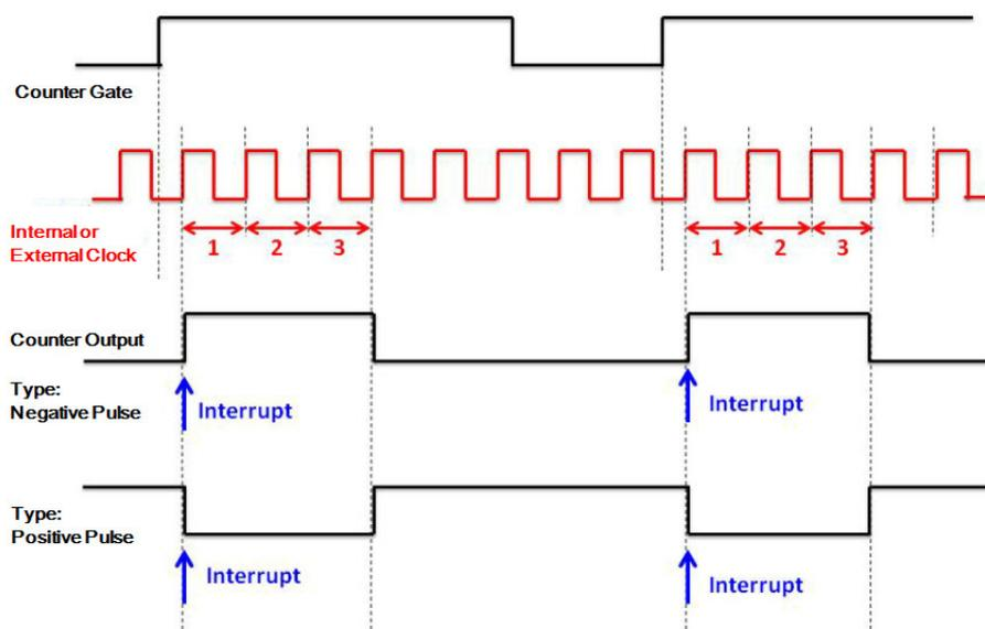
6. PWM Output: PCIE-1816/1816H can generate PWM (pulse width modulation) signal which you can configure its logic high time and logic low time as figure below. The available period range for logic high time and logic low time is 100 ns ~ 214 second.
