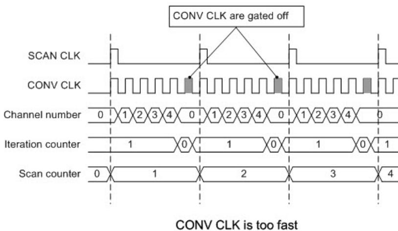
Other scanning procedure applications timing diagram.
