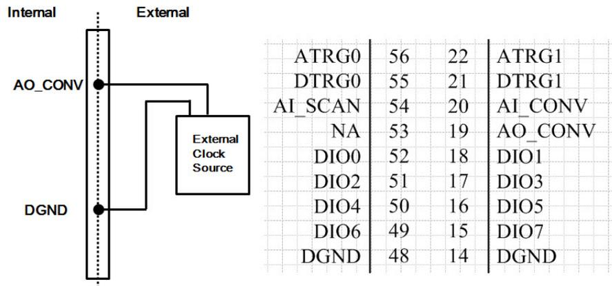
Figure 3.10 External Clock Source Connection
