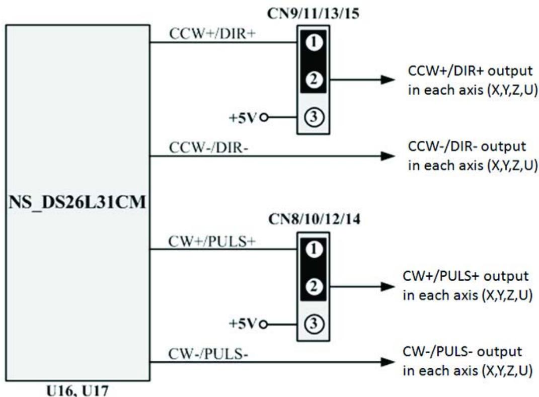
**Figure 3.3 Pulse out Signal Diagram**
