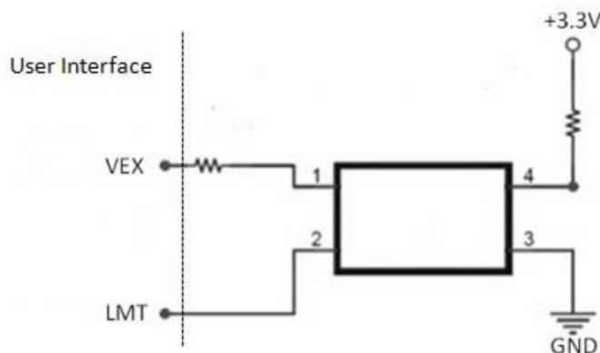
Figure 3.6 Circuit Diagram for Limit Input Signals
