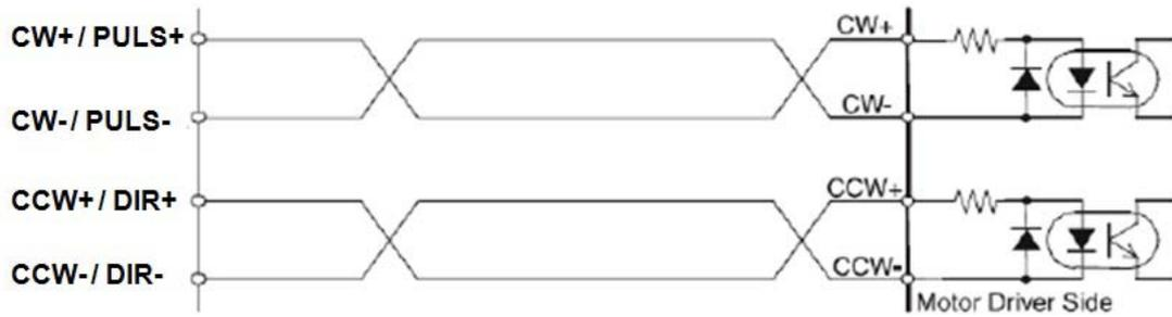
**Figure 3.4 Photocoupler Interface**
