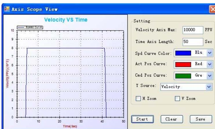
Wherein, on the right there are setting and operating buttons, on the left there is movement/speed curve in single-axis motion.
