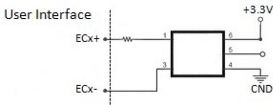
Figure 3.7 Circuit Diagram of Encoder Feedback
