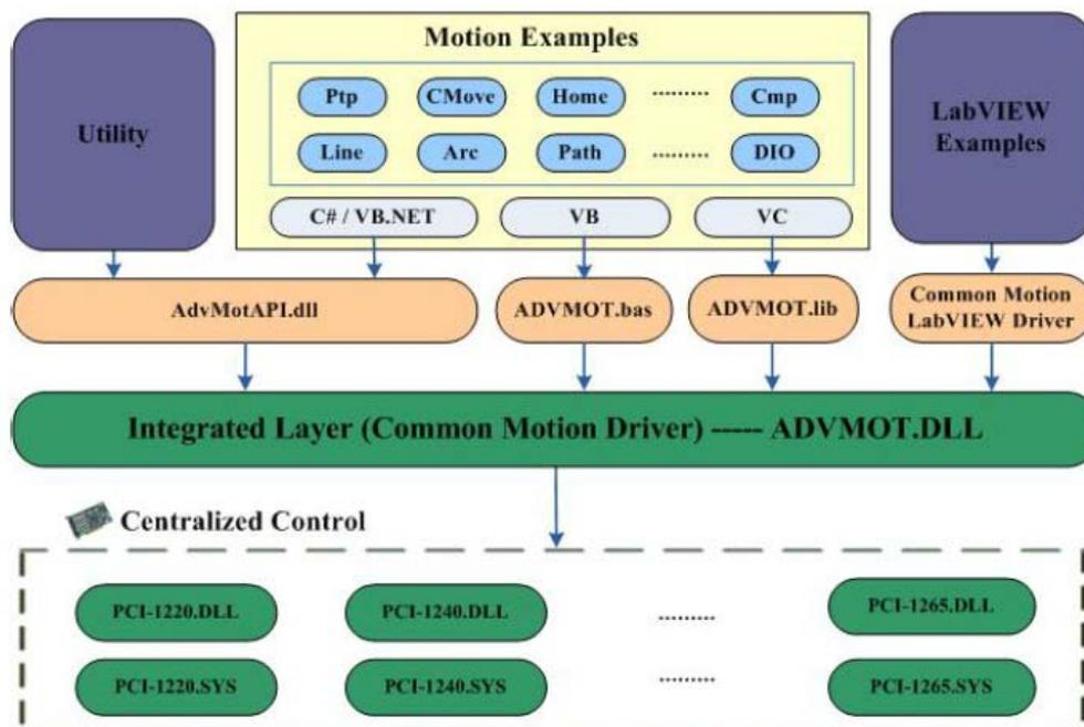
Figure 6.1 PCI-1245L Software Architecture
