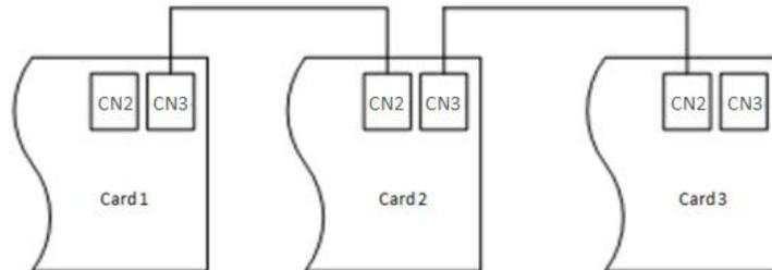
**Figure 3.9 Connection of Multiple Cards**
