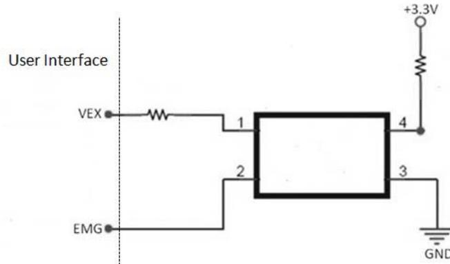
**Figure 3.8 Circuit Diagram of Emergency Stop Input Signal**
