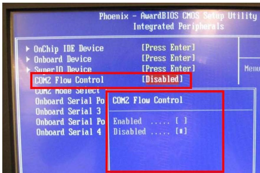
Step 4. Into the " **Integrated Peripherals** " page, index to move to " **COM2 Mode Select** ", then press "Enter" key.
