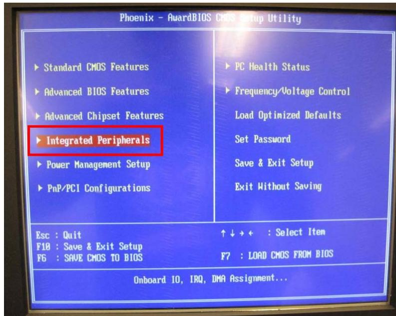
Step 3. Into the "**Integrated Peripherals**" page, index to move to "**COM2 Flow Control**", then press "**Enter**" key.
