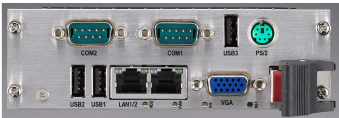
Figure 1.4 MIC-3325 8HP front panel ports, indicators and buttons
