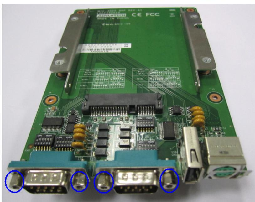
11. Fix the XTM board on the 4HP motherboard.
