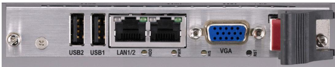
Figure 1.3 MIC-3325 4HP front panel ports, indicators and buttons
