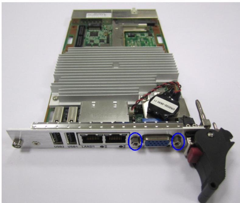
2. Remove two screws on the bottom side.
