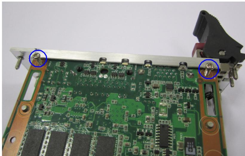
9. Install four posts with M2.5\*5L screws on the bottom side.
