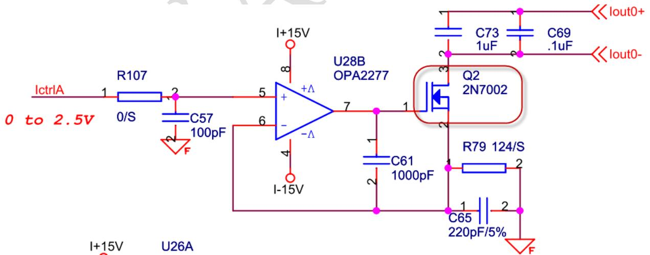
Take the picture above to explain the situation more clearly, the output of the current is controlled by the MOSFET (Q2) in the picture.
