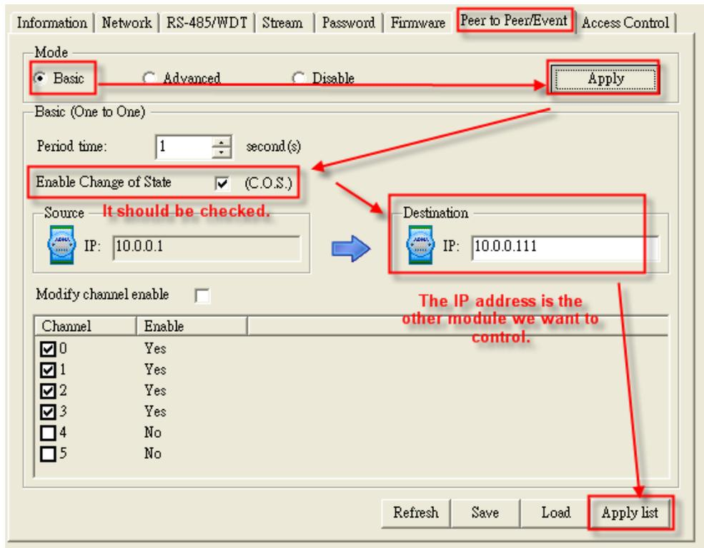
6. You could set the other module in the same way. If you don't want the opposite module to control the near module, just don't change the setting in the Peer to Peer/Event tab.
